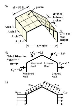
*Hint*: The load on each arch segment (wall or roof) can be estimated using a basic load-distribution model. The *tributary area* on each arch segment – the area contributing to its load – is half the wall or roof area that the arch segment shares with the neighboring arch(es).
