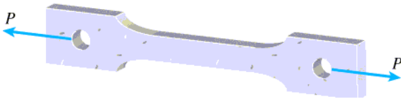
Figure 1.2a Axial member in tension.
